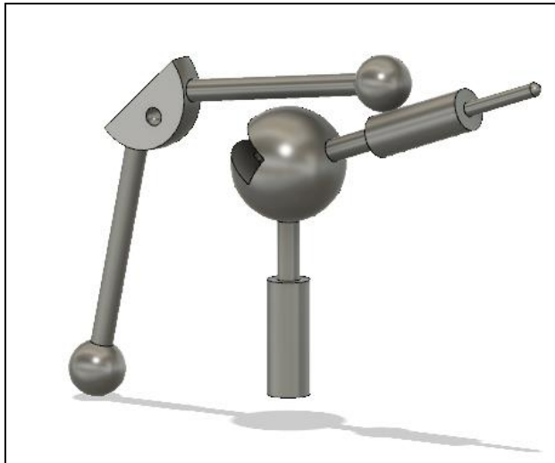
Figure 11. CAD model of the two pieces which snap together to make one polyethylene monomer. The initial sketch for the piece on the left is shown in Figure 12.
